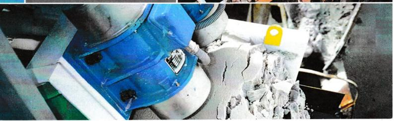
Dewatering Screens reduce water content in the final product to a minimum value, depending on the characteristics of the sand and its natural water absorption coefficient or degree of saturation. Eral UK offers a wide range of equipment sizes, in order to achieve high product quality expectations from operators.
