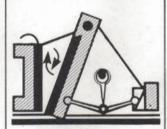
Blake double toggle crushers waste power. Pitman is in tension, swinging jaw is lifted and crushing is a combination of compression and attrition.
