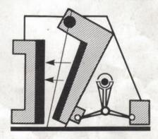
Our crushers are so finely balanced that they can be turned over by hand. They operate faster and last longer as they crush by pure compression
